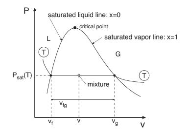
$$egin{array}{lll} u &=& (1-x)u_f + x \ u_g = u_f + x \ u_{fg} \Rightarrow x = rac{u-u_f}{u_{fg}} \ \\ h &=& (1-x)h_f + x \ h_g = h_f + x \ h_{fg} \Rightarrow x = rac{h-h_f}{h_{fg}} \ \\ s &=& (1-x)s_f + x \ s_g = s_f + x \ s_{fg} \Rightarrow x = rac{s-s_f}{s_{fg}} \end{array}$$
