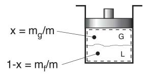
total mass of mixture  $\Rightarrow m=m_g+m_f$  mass fraction of the gas  $\Rightarrow x=m_g/m$  mass fraction of the liquid  $\Rightarrow 1-x=m_f/m$
