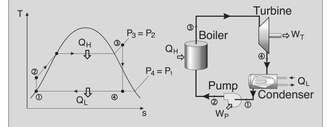
find:  $\dot{Q}_H, \dot{Q}_L, \dot{W}_{net} = \dot{W}_T - \dot{W}_P$ , and the overall cycle efficiency,  $\eta_R$  given the following conditions:
