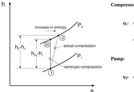
Work Input Devices: i.e. Compressors and Pumps
