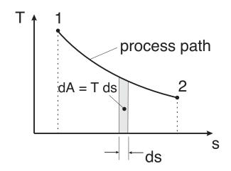
• the area under the curve on a T-s diagram is the heat transfer for internally reversible processes
