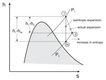
Work Output Devices: i.e. Turbines and Nozzles
