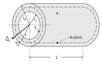
Steady, 1D heat flow from  $T_1$  to  $T_2$  in a cylindrical system occurs in a radial direction where the lines of constant temperature (isotherms) are concentric circles, as shown by the dotted line and T = T(r).
