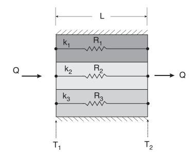
$$\dot{Q}_1=rac{T_1-T_2}{R_1} \qquad \qquad R_1=rac{L}{k_1A_1} \ \dot{Q}_2=rac{T_1-T_2}{R_2} \qquad \qquad R_2=rac{L}{k_2A_2} \ \dot{Q}=\sum \dot{Q}_i=(T_1-T_2)\left(\sumrac{1}{R_i}
