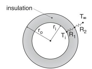
Consider a steady, 1-D problem where an insulation cladding is added to the outside of a tube with constant surface temperature  $T_i$ . What happens to the heat transfer as insulation is added, i.e. we increase the thickness of the insulation?
