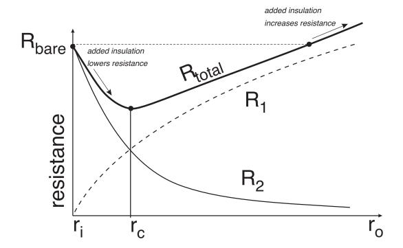
There is always a value of  $r_{cr,cal}$ , but there is a minimum in heat transfer only if  $r_{cr,cal} > r_i$
