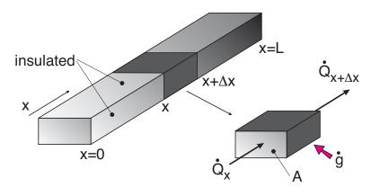
The general 1-D conduction equation is given as
