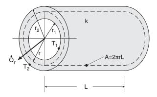
Steady, 1D heat flow from  $T_1$  to  $T_2$  in a cylindrical systems occurs in a radial direction where the lines of constant temperature (isotherms) are concentric circles, as shown by the dotted line in the figure above and T = T(r).
