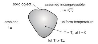
For the 3-D body of volume V and surface area A, we can use a lumped system analysis if
