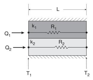
In general, for parallel networks we can use a parallel resistor network as follows:
