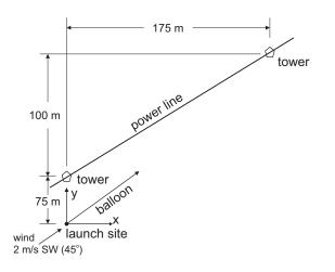
A hot air balloon is being launched from a field adjacent to a high voltage power line. As the balloon leaves the ground, a 2 m/s gust of wind from the southwest blows the balloon towards the power lines. Assume that the balloon ascends at a steady rate of 0.5 m/s and the power lines are at a constant height of 30 m (no line sag between the towers). A plan view of the launch site and the power line is shown in the figure.
