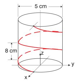
To protect a water pipe from freezing in winter temperatures, a heat cable is wrapped around the pipe. The wire is wrapped in a circular helix around the 5 cm diameter pipe with a complete turn around the pipe every 8 cm. Assume that the wire diameter is negligible.
