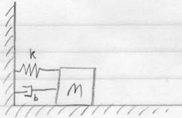
$$\begin{aligned}k &= 200 \text{ N/m} \\b &= 140 \text{ N}\cdot\text{sec}/\text{m} \\m &= 20 \text{ kg}\end{aligned}$$
