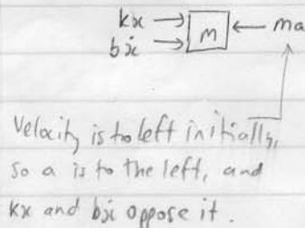
$$\begin{aligned}kx + bxi &= -m\ddot{x} \\20\ddot{x} + 140\dot{x} + 200x &= 0 \\x'' + 7x' + 10x &= 0 \\r^2 + 7r + 10 &= 0 \\(r+5)(r+2) &= 0\end{aligned}$$
