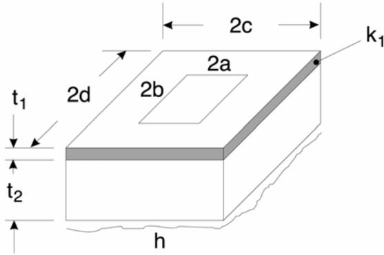
Figure 2: Test Coupon for Spreading Resistance Calculations
