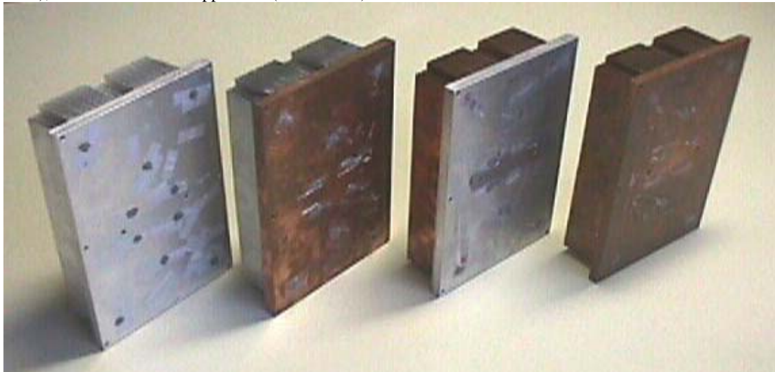
Figure 2: Tested heatsink combinations. Starting from left: Aluminum base/Aluminum fin (Al B–Al F), Copper Base/Aluminum Fin (Cu B–Al F), Aluminum base/Copper Fin (Al B–Cu F) and Copper Base/ Copper Fin (Cu B–Al F).
