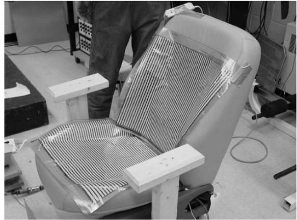
Figure 5: Covering the seat prototype with Tekscan pressure mats.
