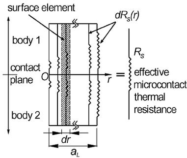
**Fig. 8 Thermal resistance network for surface elements.**
