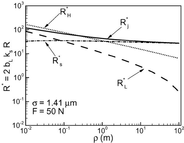
Fig. 13 Effect of radius of curvature on TCR.
