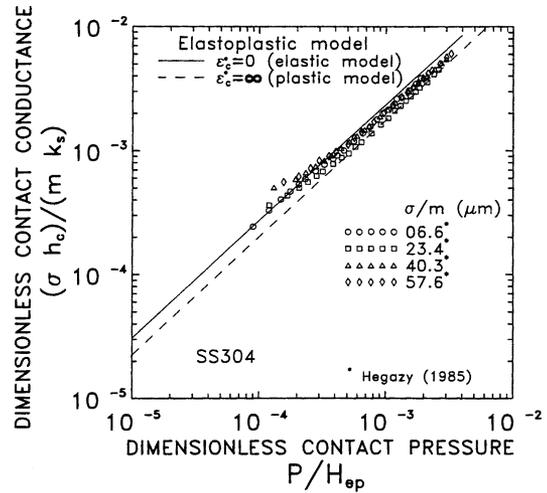
Fig. 29. SS 304 data versus elastoplastic contact conductance model.
