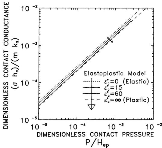
Fig. 27. Elastoplastic contact conductance model versus relative contact pressure.
