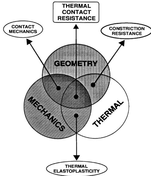
Fig. 7. Triad for thermal contact resistance (conductance).
