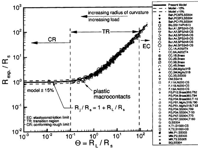
Fig. 33. Comparison of compact model with all conforming and nonconforming rough surface data.
