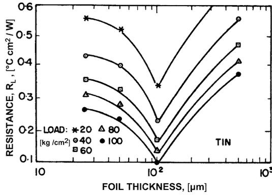
Fig. 12. Effect of tin foil thickness during first load.
