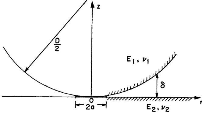
Fig. 10. Schematic of sphere-flat contact and macrogap.
