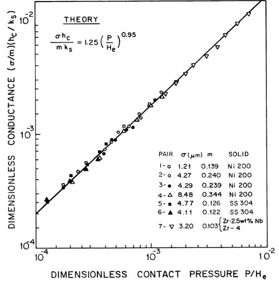
Fig. 15. Comparison of vacuum data for four metals with extended CMY model.
