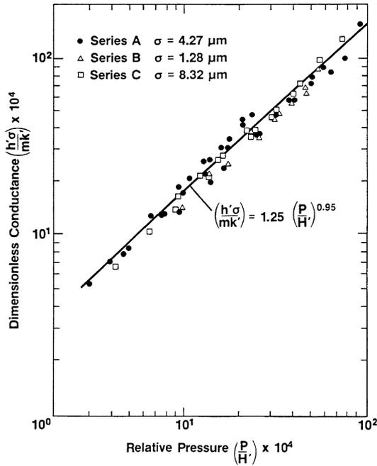
Fig. 22. Dimensionless contact conductance versus dimensionless contact pressure: all data and CMY model.
