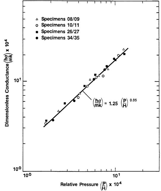
Fig. 20. Comparison of Ni 200 vacuum data and extended CMY model.
