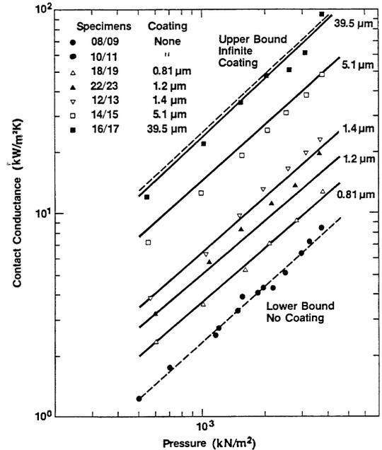
Fig. 21. Contact conductance data and model predictions versus contact pressure.
