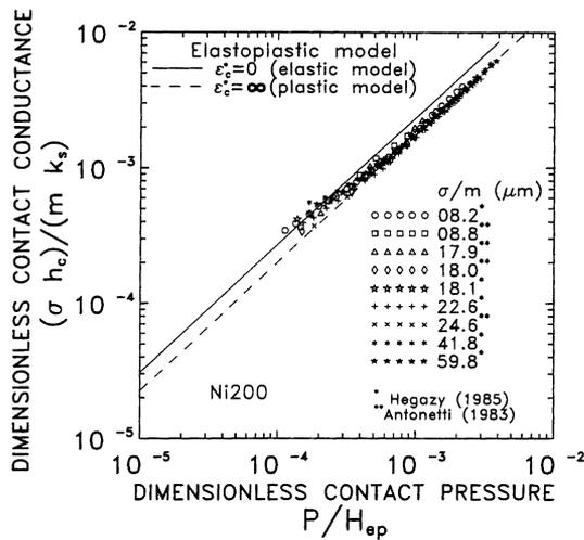
Fig. 28. Ni 200 data versus elastoplastic contact conductance model.
