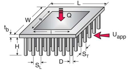
Fig. 2. Geometry of in-line pin-fin heat sink.
