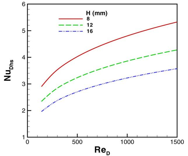
Fig. 10. Nusselt number as function of  $Re_D$  and  $H$  for in-line arrangement.
