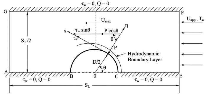
Fig. 3. Control volume for prediction of heat transfer from PFHS.
