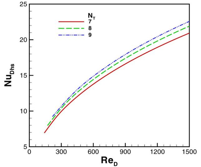
Fig. 9. Nusselt number as function of  $Re_D$  for in-line arrangement.
