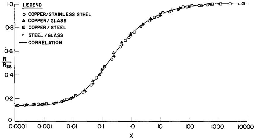
FIG. 5. Constriction resistance vs the correlation parameter  $X$ .
