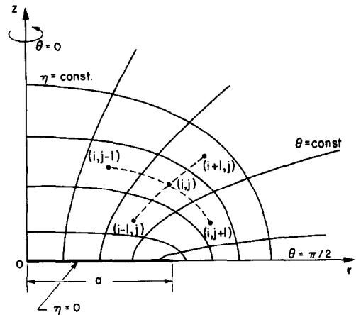
FIG. 3. Discretization of the solution domain.
