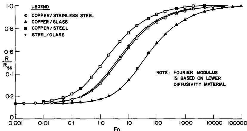
FIG. 4. Constriction resistance vs Fourier modulus based on low diffusivity material.
