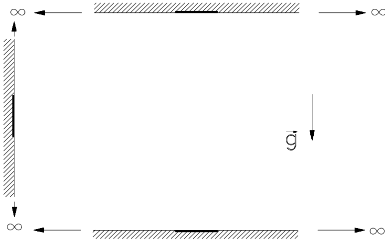
Figure 1: Schematic of Finite Isothermal Plates Embedded in Infinite Adiabatic Planes: Vertical and Horizontal Orientations.
