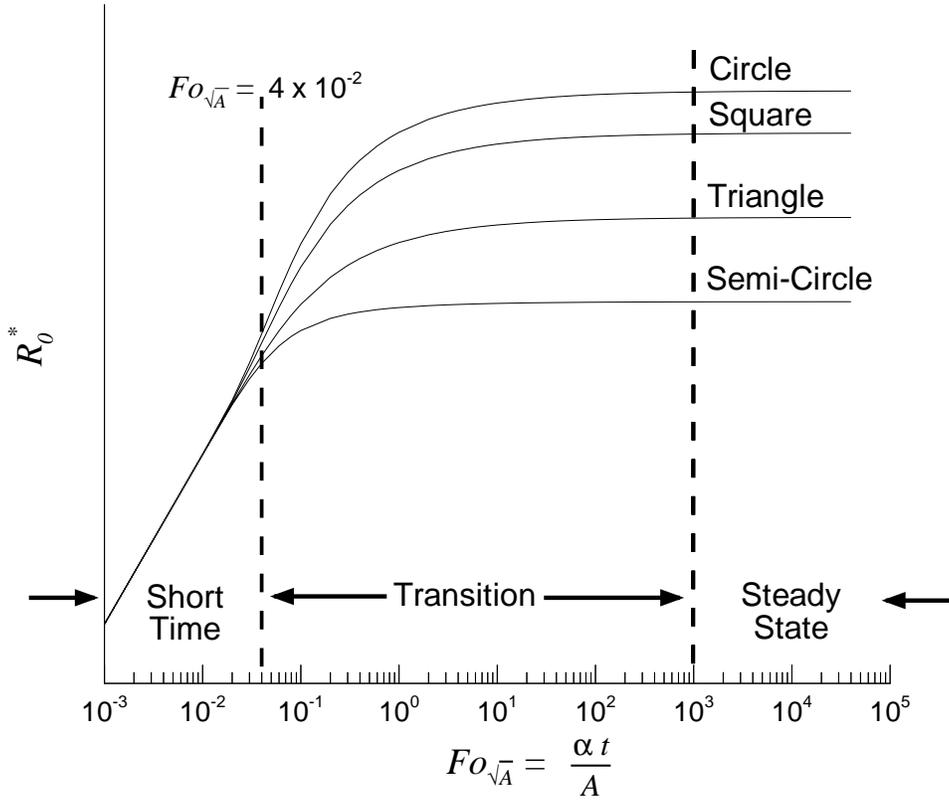
Figure 4: Diagram of Universal Time Function for Various Contact Shapes
