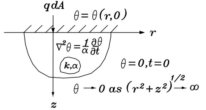
Figure 1: Point Source on Adiabatic Surface of a Semi-Infinite Body
