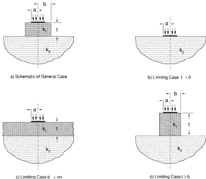
Fig. 1. Typical spreading resistance problems.
