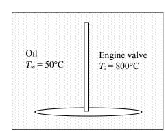
$$b = \frac{hA_s}{\rho c_p \mathbf{V}} = \frac{8h}{1.8\rho c_p D} = \frac{8(800 \text{ W/m}^2.^{\circ}\text{C})}{1.8(7840 \text{ kg/m}^3)(440 \text{ J/kg.}^{\circ}\text{C})(0.008 \text{ m})} = 0.1288 \text{ s}^{-1}$$
