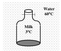
**Properties** The thermal conductivity, density, and specific heat of the milk at 20°C are k = 0.598 W/m.°C,  $\rho = 998$  kg/m<sup>3</sup>, and  $c_p = 4.182$  kJ/kg.°C (Table A-15).
