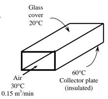
which is greater than 10,000. Therefore, the flow is turbulent and the entry lengths in this case are roughly  $L_h \approx L_t \approx 10D_h = 10(0.05825 \text{ m}) = 0.5825 \text{ m}$
