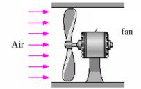
$$\dot{W}_{\text{sh, in}} = \dot{m}_{\text{air}} \frac{V_{\text{out}}^2}{2} = (4.72 \text{ kg/s}) \frac{(10 \text{ m/s})^2}{2} \left( \frac{1 \text{ J/kg}}{1 \text{ m}^2/\text{s}^2} \right) = 236 \text{ J/s} = 236 \text{ W}$$
