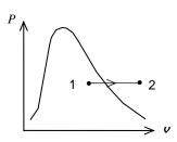
(c) At the final state water is superheated vapor, and its specific volume is
