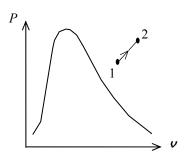
(b) The pressure of the gas changes linearly with volume, and thus the process curve on a P-V diagram will be a straight line. The boundary work during this process is simply the area under the process curve, which is a trapezoidal. Thus,
