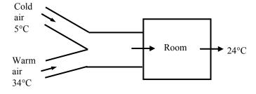
**Analysis** (a) We take the mixing chamber as the system, which is a control volume since mass crosses the boundary. The mass and energy balances for this steady-flow system can be expressed in the rate form as
