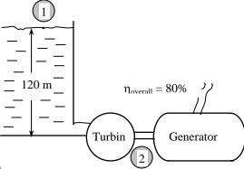
$$e_{\text{mech}} = pe = gz = (9.81 \,\text{m/s}^2)(120 \,\text{m}) \left(\frac{1 \,\text{kJ/kg}}{1000 \,\text{m}^2/\text{s}^2}\right) = 1.177 \,\text{kJ/kg}$$
