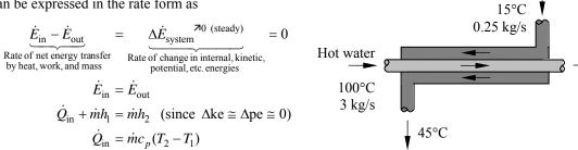
Then the rate of heat transfer to the cold water in this heat exchanger becomes
