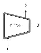
There is only one inlet and one exit, and thus  $\dot{m}_1 = \dot{m}_2 = \dot{m}$ . We take the compressor as the system, which is a control volume since mass crosses the boundary. The energy balance for this steady-flow system can be expressed in the rate form as
