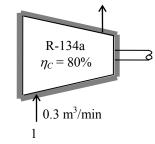
$$\eta_{c} = \frac{h_{2s} - h_{l}}{h_{2a} - h_{l}} \longrightarrow h_{2a} = h_{l} + (h_{2s} - h_{l})/\eta_{c} = 236.97 + (281.21 - 236.97)/0.80 = 292.26 \text{ kJ/kg}$$
