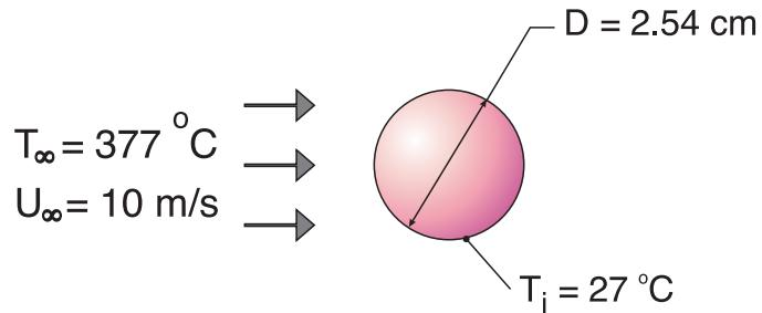
The fluid properties are calculated at the ambient temperature,  $T_\infty = (377 + 273) \text{ K} = 650 \text{ K}$
