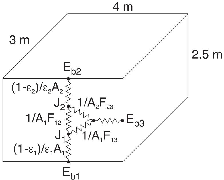
Modelling the room as a three-surface enclosure with one surface re-radiating, the heat loss equation is given as
