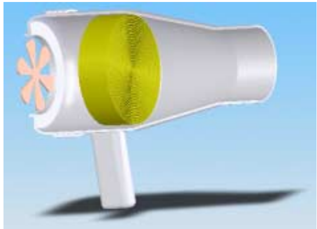
Cross-section of hair dryer showing heating element and fan
