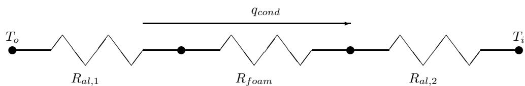
$$\begin{aligned} q_{cond} &= \frac{T_o - T_i}{R_{eq}}, \\ R_{eq} &= R_{al,1} + R_{foam} + R_{al,2}. \end{aligned}$$
