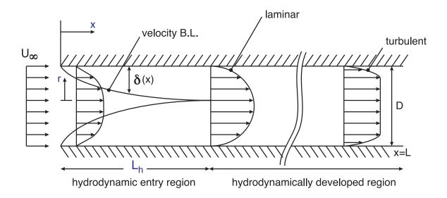
The velocity profile across the tube changes from U=0 at the wall to a maximum value along the center line. The average velocity, obtained by integrating this velocity profile, is called the *mean velocity* and is given as
