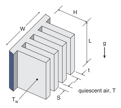
For a given baseplate area,  $m{W} imes m{L}$ , two factors must be considered in the selection of the number of fins
