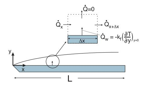
Performing an energy balance over a control volume of width  $\Delta x$  and height  $\delta_T$ , as shown above we obtain
