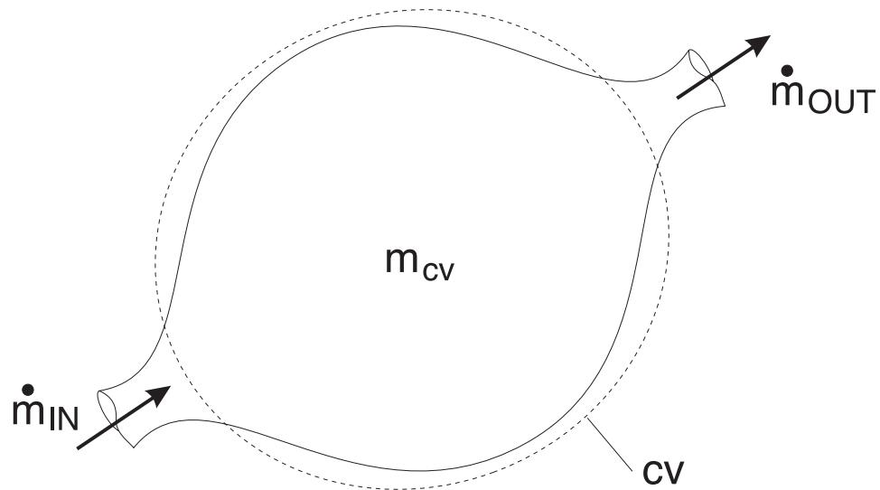
$$\left\{ \begin{array}{l} \text{rate of increase} \\ \text{of mass within} \\ \text{the CV} \end{array} \right\} = \left\{ \begin{array}{l} \text{net rate of} \\ \text{mass flow} \\ \text{IN} \end{array} \right\} - \left\{ \begin{array}{l} \text{net rate of} \\ \text{mass flow} \\ \text{OUT} \end{array} \right\}$$
