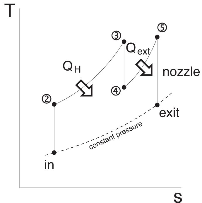
By performing a 1st law energy over the nozzle we can obtain an expression for the exit velocity in terms of the entrance temperature to the nozzle.
