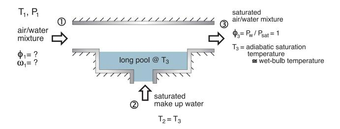
• the adiabatic saturator is used to measure humidity
