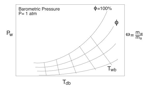
where the **dry bulb** temperature is the temperature measured by a thermometer place in the mixture and the **wet bulb** temperature is the adiabatic saturation temperature.
