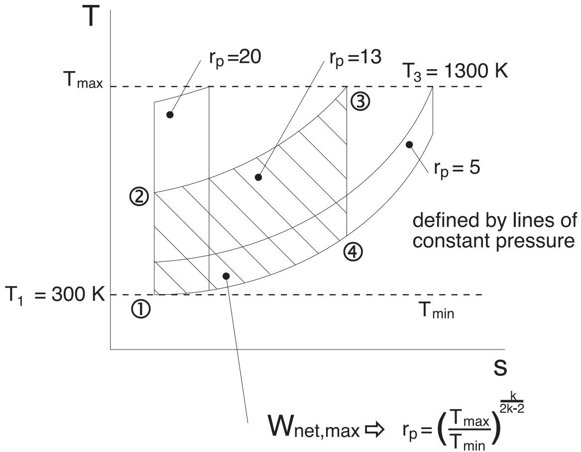
The **maximum temperature** in the cycle ( $T_3$ ) is limited by metallurgical conditions because the turbine blades cannot sustain temperatures above 1300 K. Higher temperatures (up to 1600 K can be obtained with ceramic turbine blades). The **minimum temperature** is set by the air temperature at the inlet to the engine.
