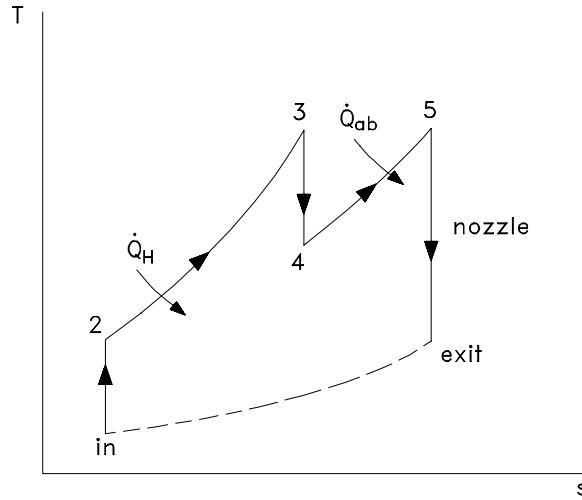
By performing a 1st law energy over the nozzle we can obtain an expression for the exit velocity in terms of the entrance temperature to the nozzle.
