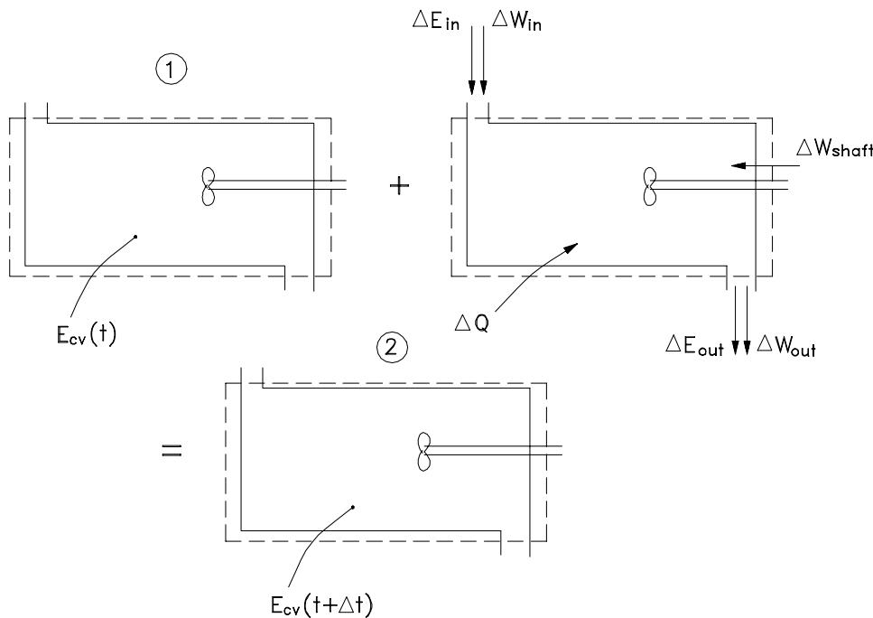
$$E_{CV}(t + \Delta t) - E_{CV}(t) = \Delta Q + \Delta W_{shaft} + \Delta m_{in}(e + Pv)_{in} - \Delta m_{out}(e + Pv)_{out}$$
