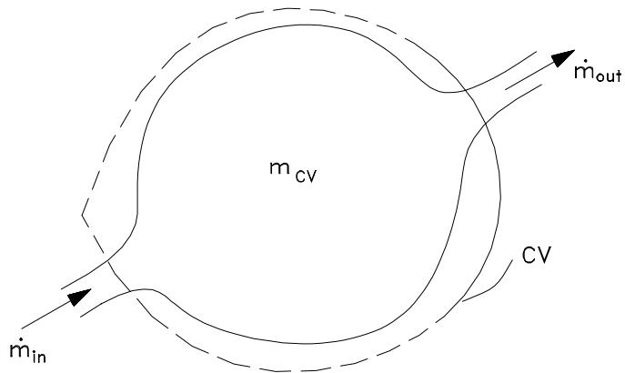
$$\left\{ \begin{array}{l} \text{Rate of Increase} \\ \text{of mass within} \\ \text{the CV} \end{array} \right\} = \left\{ \begin{array}{l} \text{Net rate of} \\ \text{mass flow} \\ \text{IN} \end{array} \right\} - \left\{ \begin{array}{l} \text{Net rate of} \\ \text{mass flow} \\ \text{OUT} \end{array} \right\}$$
