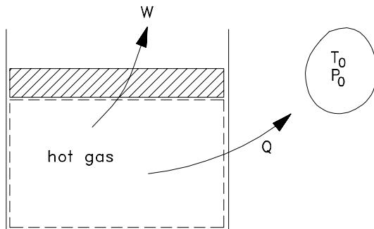
$$W_{sur} = P_0(V_2 - V_1)$$
