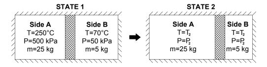
Step 1: Draw a diagram to represent the system showing control mass/volume of interest.
